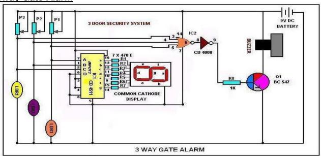
This is a zonal security system which displays the zone when trespassed by the intruders. The circuit has a seven segment display indicating the gate number.
